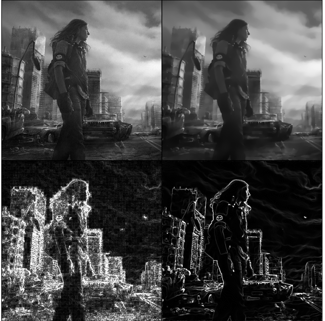
Fig. 5. Top left: Original image (source: www.fishki.net ). Top right 2 x 2 pixel scheme for total variation diffusion, \tau = 5 \times 10^{-4} , 100 iterations. Bottom left: Fuzzy edge detector. Original image. Bottom right: Fuzzy edge detector. Filtered image. Author: S. Kosov (2006)
