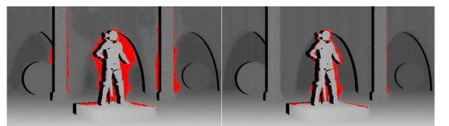
Comparison of the average percentage of bad pixels for the dynamic scene with AI scene (error threshold = 1 pixel). Improvement ratio are given in brackets:
